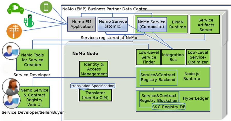
**Fig. 2.** The components deployed to a NeMo node
