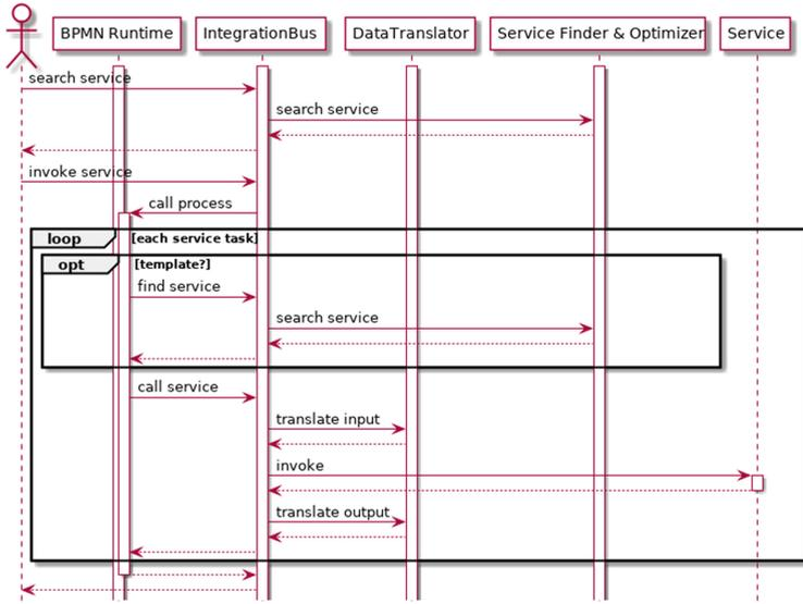
Fig. 5. Sequence diagram of the workflow, slightly simplified.
